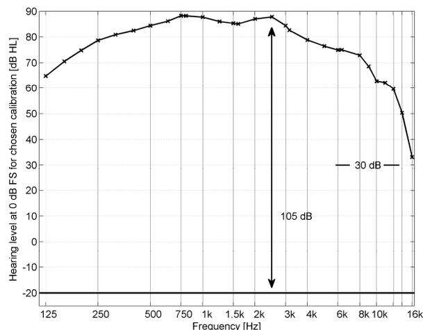
Figure 4 Measured reference threshold of hearing for headphone HDA-200 at 0 dB FS output of sound card
