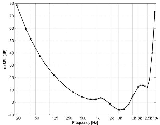
Figure 3 Reference threshold of hearing for free-field pure tone audiometry, as defined in ISO 389-7:2005 [8]
